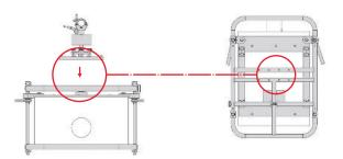
Place the truss mount on the rear side of the frame. Make sure that the 8 screws enter the 8 holes in the frame. Tighten the screws to secure the truss mount on the frame.
