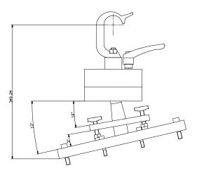
The distance between the two C-clamps is variable adjustable within a range of 40 mm. Make sure that the screws are properly tightened after setting a bolting torque of 34 Nm.
